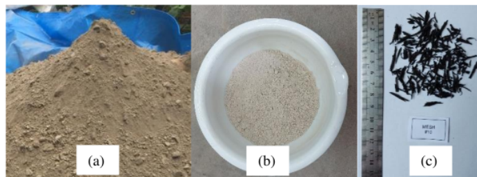
Figure 1. Material used, (a) Dredged soil; (b) Trass; and (c) Shredded tires
